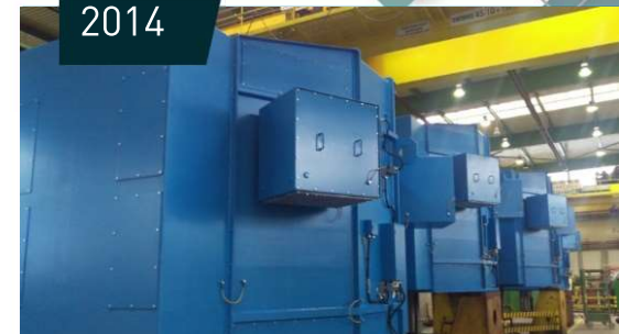
ROSTOV 4 NPP, Russia FVDZ1126 V20, FVDZ 1126V22 (3x 3300 kW, 6kV, 300 rpm) (4x 4500 kW, 6kV, 272 rpm)
