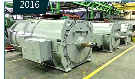
SWCC Saudi Arabia, IP65 FOC 710Ls6 (6x 1950 kW, 6.6 kV 1000 rpm)
