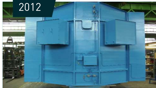
ROSTOV 3 NPP, Russia FVDZ1126 V20, FVDZ 1126V22 (3x 3300 kW, 6kV, 300 rpm) (4x 4500 kW, 6kV, 272 rpm)
