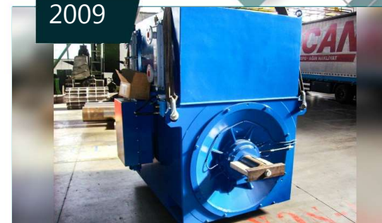
EUAS - KANGAL PP, Turkey, FBDZ 566L4 (1700 kW, 6 kV, 1481 rpm) FBDz 716 L12 (1250 kW, 6 kV, 493 rpm)
