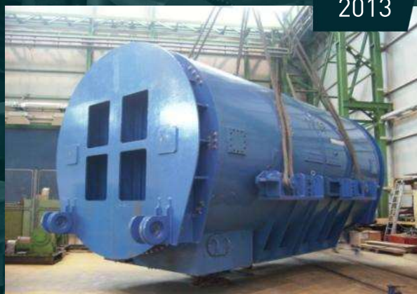
Paks Nuclear Power Plant, Hungary Stator rewinding & refurbishment of TVV-221 type 250 MVA, 3000 rpm turbogenerator
