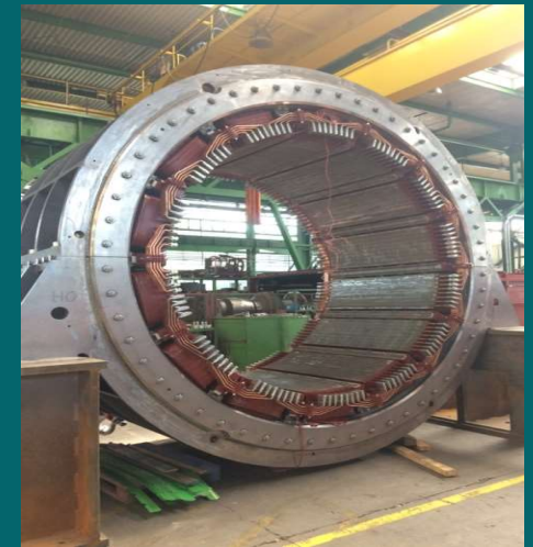
Stator manufacturing & rotor refurbishment of P23/165-4.6 type 4600 kW 50/90 rpm DC motor, 2015 Weight 200 tons
