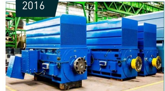
FIVES FCB D'Ech Cheliff Cement, Algeria FDDRp 903L24 (2x 1150 kW, 3300 V, 248 rpm)
