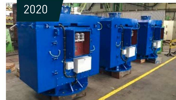
Kudankulam NPP, India FTCV 400Jv4 (18x 2000 kW, 6kV, 1490 rpm)
