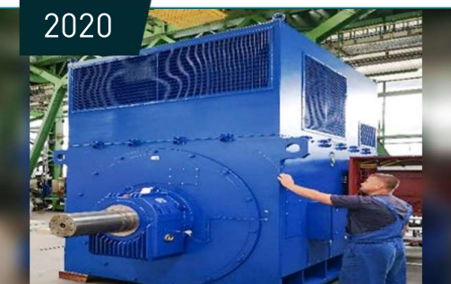
HPP Xeset, Lao PDR 2x 5795 kVA, 12P, 11 kV, 500 rpm Francis
