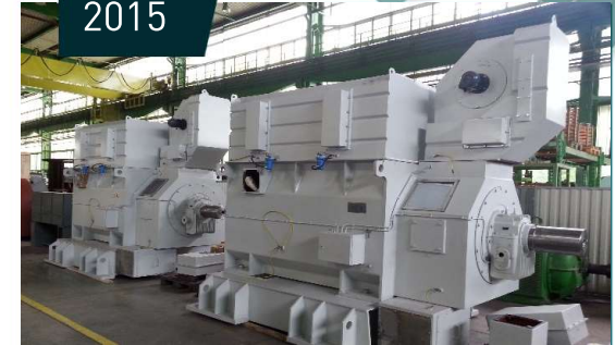
MEFTAH Lafarge Cement plant, Algeria FRA 710Hm8 (2x 3300 kW, 5500 V, 744 rpm)
