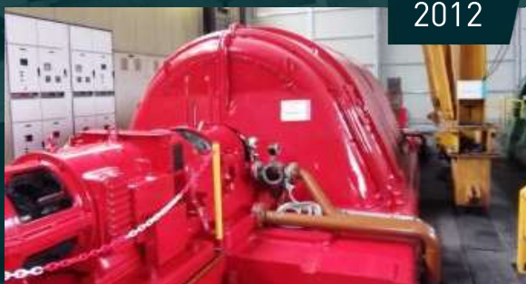
ABB Sace, Bergamo Italy Generator rotor overhauling – retaining rings changing ( 50 Hz – 60 Hz )- English Electric, 80 MVA Type: TG 40-220-87
