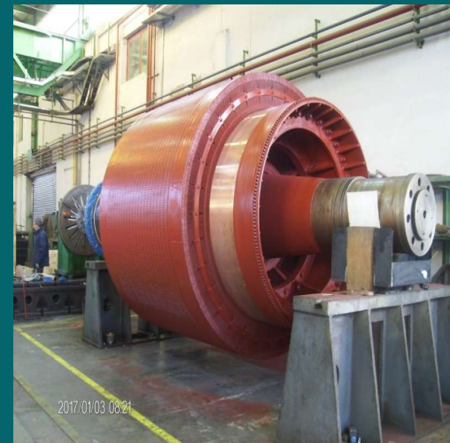
Stator manufacturing & rotor refurbishment of P23/165-4.6 type 4600 kW 50/90 rpm DC motor, 2015 Weight 200 tons
